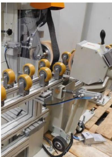
Pneumatically supported contact wheel & BA
